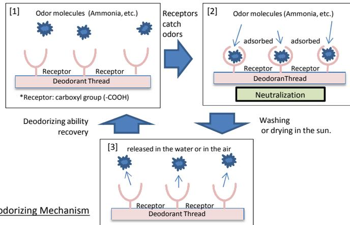
[Fig-2] Deodorizing Mechanism
